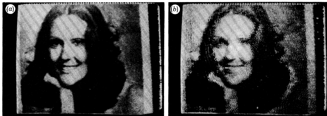
FIGURE 6. Television original (a) and image (b) after transmission through 2000 m of water (C.N.E.X.O.).
